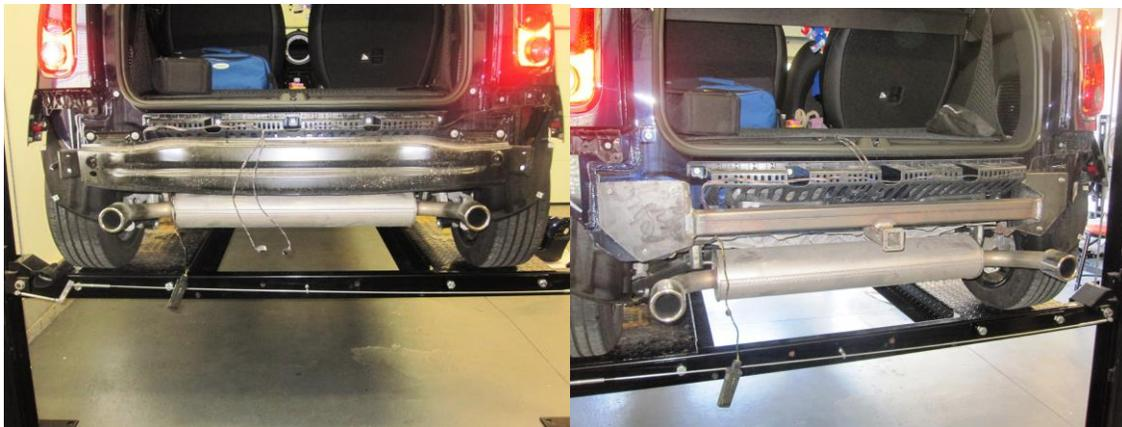
Remove the six 17mm bolts holding the steel bumper substructure to the car.
